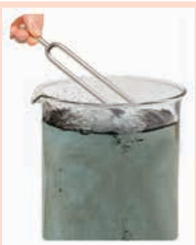
Tip of a vibrating tuning fork produces disturbances on water surface
