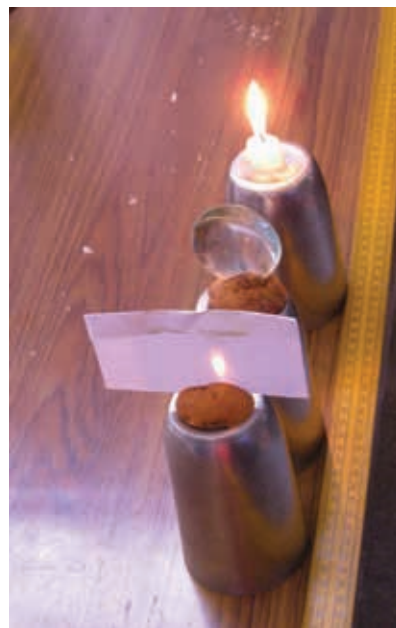
Improvisation for finding focal length of a convex lens
