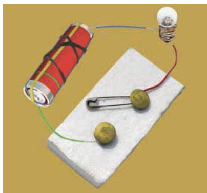
An improvised electric switch
