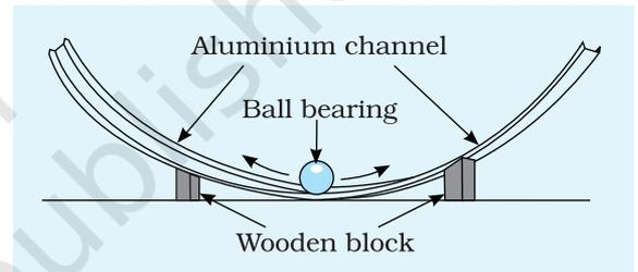
**Fig. D 15.6:** Arrangement to demonstrate the to-and-fro motion of a steel ball in a channel in the form of an arc of a circle
