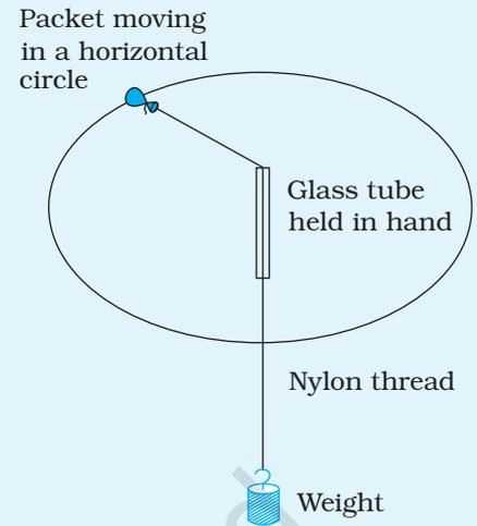
**Fig. D 3.2:** On revolving the packet of sand at a suitable speed, the weight lifts off the table; its weight is just enough to provide the necessary centripetal force
