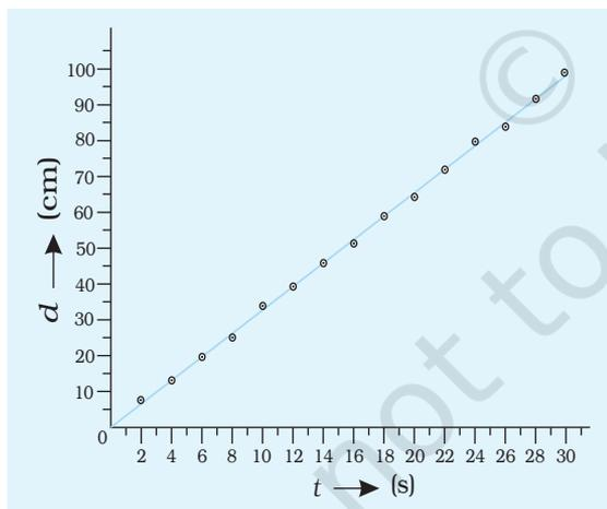
**Fig. D 1.1(c):** Distance–time graph for motion of metal ball in glycerine
