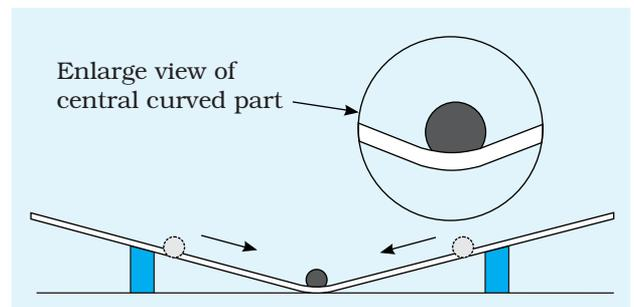
**Fig. D 15.7:** Arrangement to demonstrate the to-and-fro motion of a ball along a double inclined track
