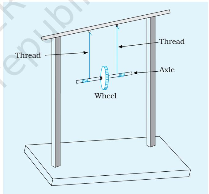
**Fig. D 5.1:** The Maxwell's wheel
