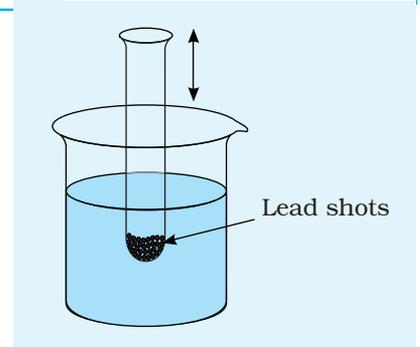
**Fig. D 15.5:** A test tube floating in vertical position due to a load in it, oscillates up and down, when it is pushed a little and then released
