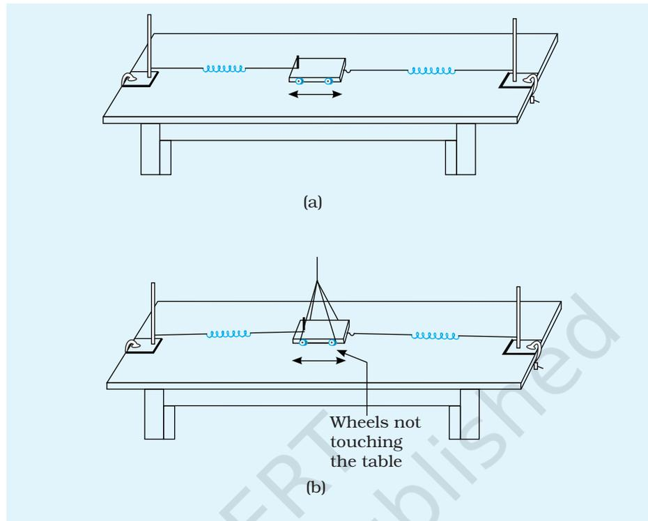
**Fig. D 15.8:** (a) Set up for demonstrating the to-and-fro motion of a trolley held between two identical springs
