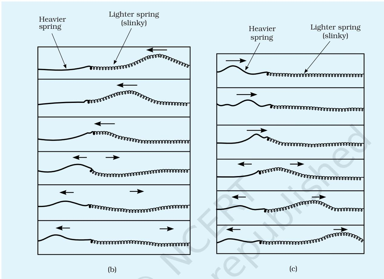
**Fig. D 19.1 (b):** Reflection and transmission of a pulse moving from a rarer medium to a denser medium
